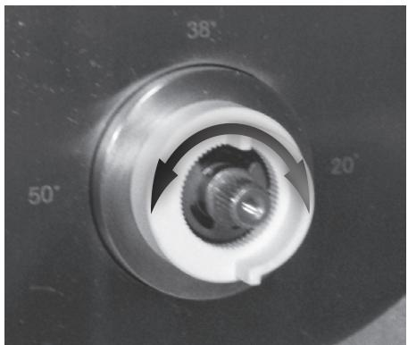
11. Use a thermometer to measure the temperature of the jet of water produced by the shower. Place the thermometer in the jet of water and adjust the thermostat, turning it counterclockwise to raise the temperature, and clockwise to reduce the temperature, until the desired temperature of 38°C / 100°F is reached.
