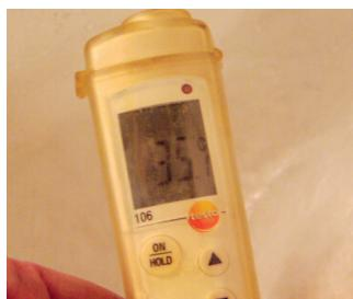
**3. Use a thermometer to measure the temperature of the jet of water produced by the shower. If the temperature of the water is not 38°C, continue to step 4**
